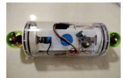
The two-propeller underwater robot
