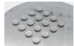
SLM-Fabricated Fe-Based Metallic Glass Samples with Re-Scan
