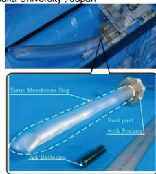
Underwater-Driven Torus-Type Buoyancy Control Mechanism
