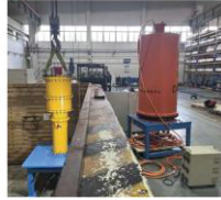
Subsea valve electric actuator test bench
