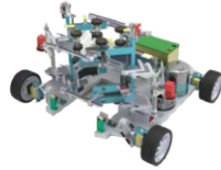
Prototype of the Separable Tree-Climbing Robot
