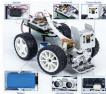
Comprehensive hardware of PiCar-X chassis and parts
