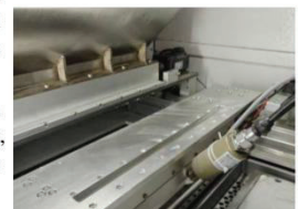
BJAM powder spreading mechanism
